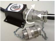
2. Connect the dust protection caps of the ISOBUS plug and the ISOBUS socket:
