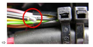
9. Insulate the soldered cable with the heat-shrink tubing.
