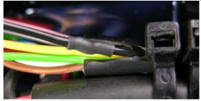
**10.** Remove the blind plug from pin 5 of the ISOBUS rear socket. If the blind plug is not visible, it may have slid in. Use for example a wire to push the blind plug from the front towards the rear.
