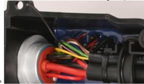
**3.** Insert the black cable that was removed from the casting compound into the insulation-displacement connector up to the stop.
