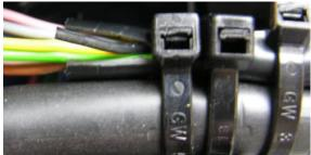
**6.** Carefully remove the insulation from the black cable line.
