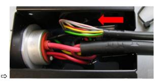
**4.** Carefully cut away approx. 2cm of the sheath until you can see the black cable line. Be careful when doing this not to damage the cable line inside.
