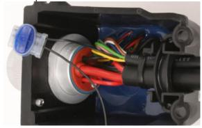
**6.** Remove the blind plug from Pin 5 of the rear ISOBUS socket. If the blind plug is not visible, it might have slipped in. Use e.g. a wire to push the blind plug through from the front to the rear.
