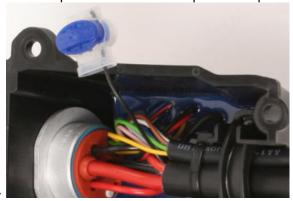
**4.** Insert the supplied "black cable with crimp contact" into the insulation-displacement connector up to the stop.
