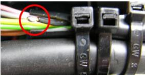
**8.** Solder the cable with crimp contact to the exposed wire. Under no circumstances use a clamp block, as the connection will not be air-tight.
