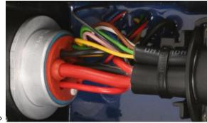
2. Remove the black cable from the casting compound.
