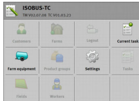
Configuration for work without ISO-XML tasks; The Taskdata folder is not on the SD card.
